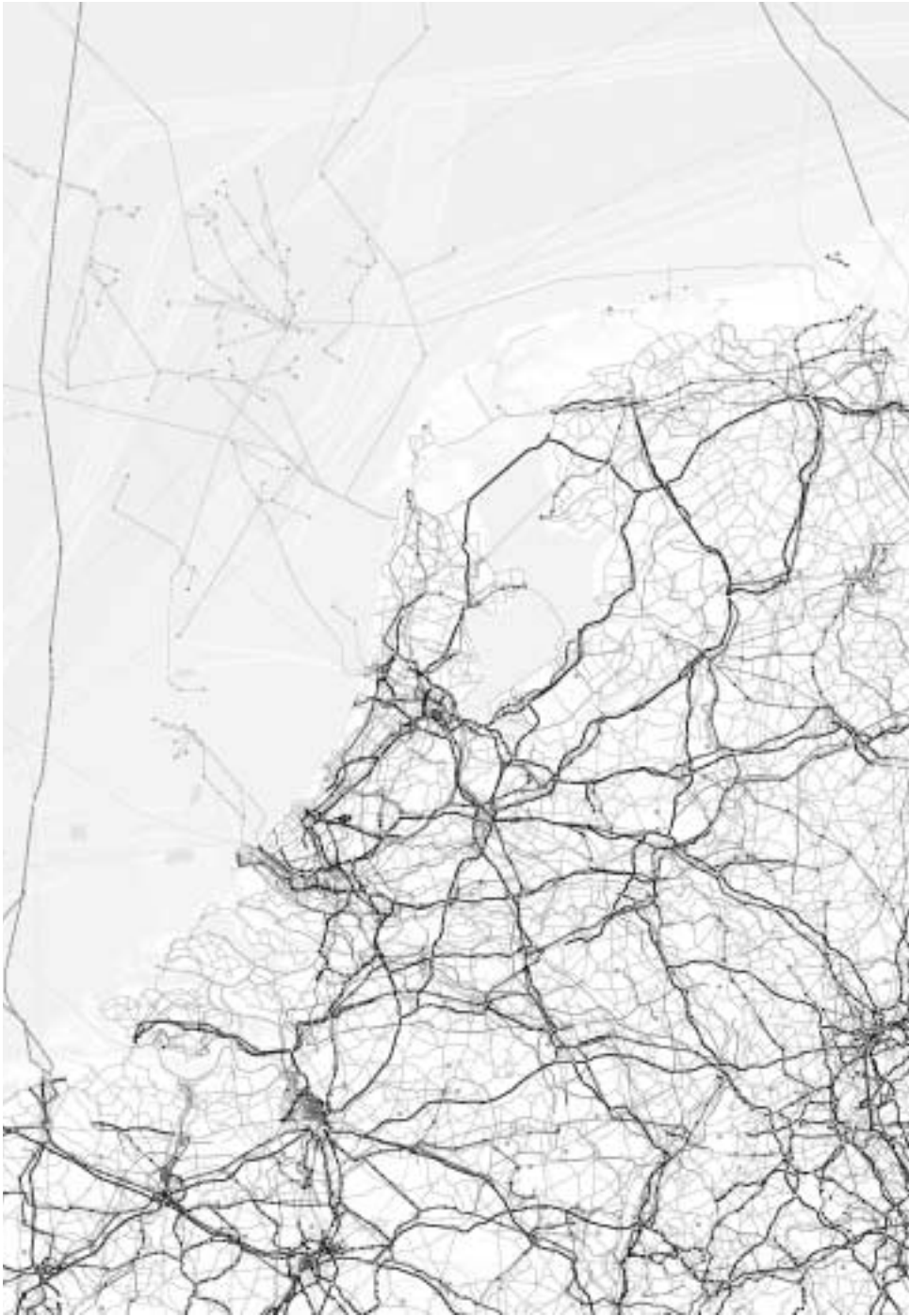
Figure 2 Around 2000 the Dutch Networked Nation was Integrated by Multiple Network Technologies. The map includes maritime and inland waterways, railways, roads, air corridors, gas pipes, oil pipes, electric power lines, and digital ICT junctions. Source: Ministry of VROM, Fifth national policy document , supplement.
